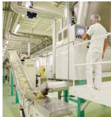
The company has seen a rise in demand for its white chocolate products. Here, a second pre-refiner sends white chocolate mass to a series of five-roll refiners.
