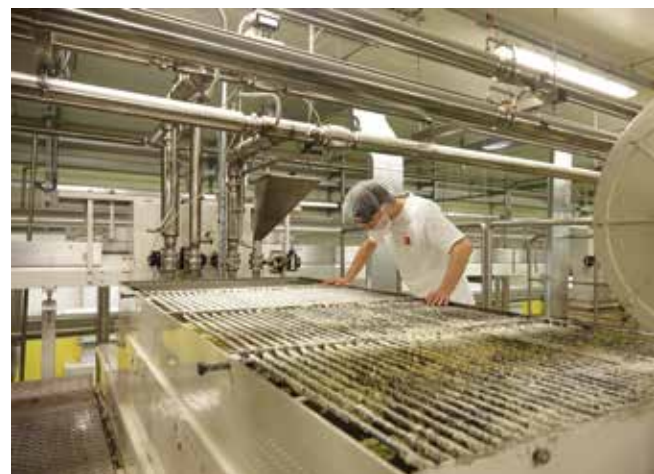
A production worker inspects conching of white chocolate. The company has seven conches that typically process chocolate from 8 to 12 hours.
