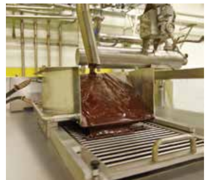
Chocolate is deposited onto a chocolate chips production line.
