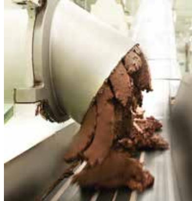
A pre-refiner sends cocoa mass toward a series of five-roll refiners for initial processing.
