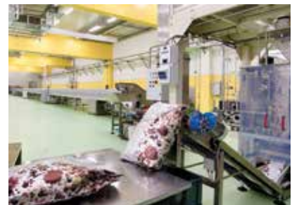
An automated bagger handles chocolate chips as they come off the line.
