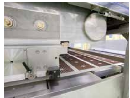
A 1.5-meter wide depositor turns out a high volume and broad range of chocolate couvertures.
