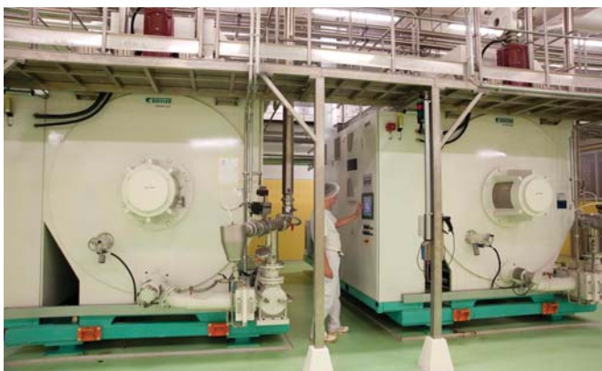
The first two of eight conches will supply finished chocolate to four moulding lines for a variety of products. The first of three cocoa presses will handle cocoa powder and cocoa butter production needs.
