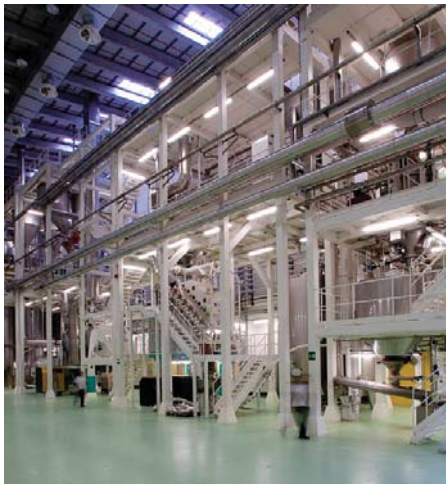
(From l. to r.) The new facility in Orsenigo features the largest cocoa bean processing complex, which includes a three-story roasting, mixing and grinding complex.
